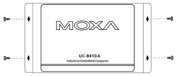
These four screws are not included in the wall-mounting kit and must be purchased separately. Refer to the detailed specifications on the right. Head Type: round or pan Head Diameter: > 4.5 mm Length: > 4 mm Thread Size: M3 x 0.5 mm
