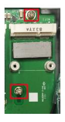
2. Remove the two silver screws 3. Install the Wi-Fi module in the socket and fasten two black screws on the module. Also, fasten the two bronze screws on the board.
