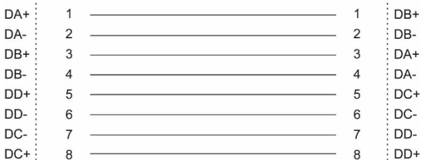
Straight-through Cable Wiring (MDI to MDI-X)
